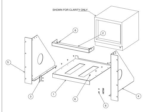
Figure 1. RMA14S Rack Mount Kit Assembly
